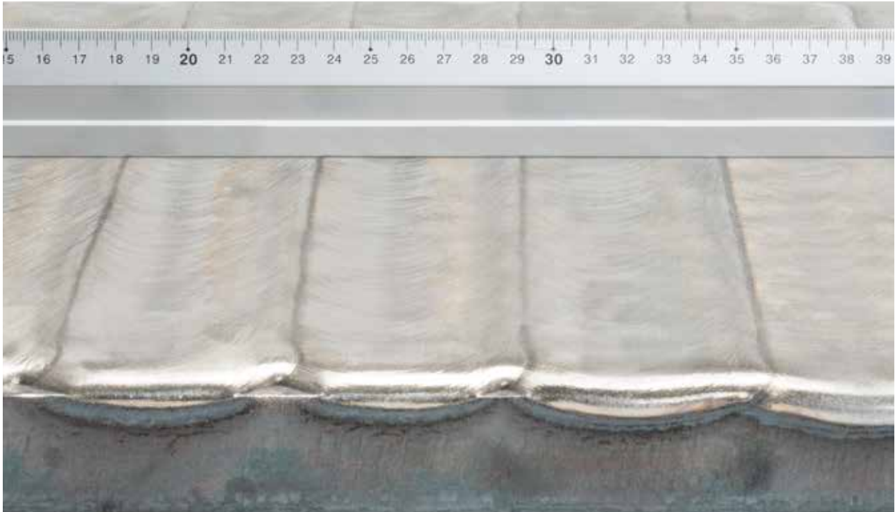
S355JR base material with a single layer Alloy 625 overlay, clad with the new strip / flux combination SOUDOTAPE 625 / RECORD EST 625-1 LD. Flat beads and smooth overlaps require minimal machining.
