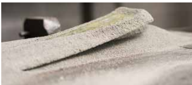
Figure 5: Cladding with RECORD EST 625-1 LD: self-releasing slag.
